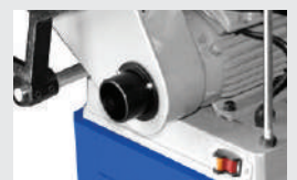
Dust collector port
