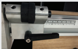
Adjustable X and Y Axis Flip Stops
