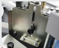
Tape Guide Ensure the alignment between the tape and workpiece.
