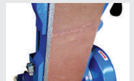
Tiltable belt from 0° to 90°
