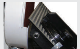
Tiltable table from 0° to 45°
