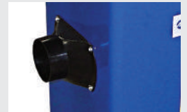
Entry to dust collector
