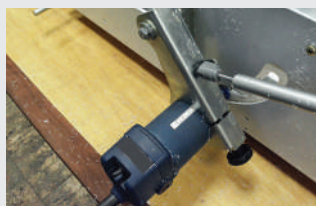
Trimmer positioned in RBB.1000
